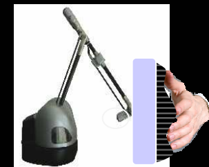
Haptic device on a 6-degree of freedom robot arm
